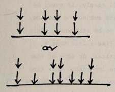
Vertical continuity. If the corners of spaces are most critical, and thickest, then these corners must be vertically continuous just as columns are in a conventional structure.
