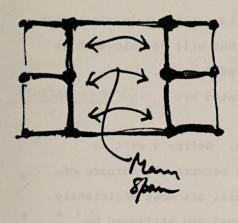
Each corner will either be a three or four way corner. This follows directly from postulate 8. A five way corner would create at least one acute angled space. If the connection is four way, it has to be right angled, to meet postulate 11. This means there are essentially three kinds of valid interior corners, in plan.
