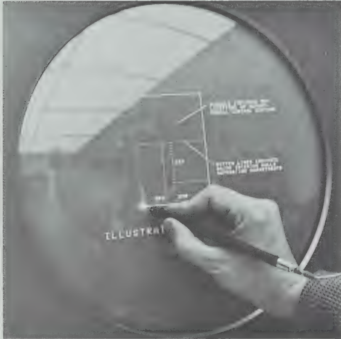
1. Sketching with a light pen on a computer oscilloscope screen to introduce a schematic plan into computer memory. 2
