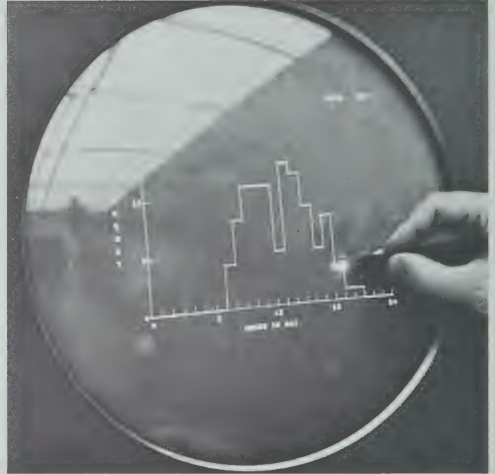
3. Entering a site plan into computer memory by tracing with a graphic input device. 3 The plan is displayed on the counter oscilloscope as drawn, and labels are added by typewriter. 4
